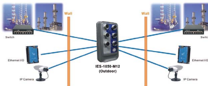
Connections of Ethernet devices
